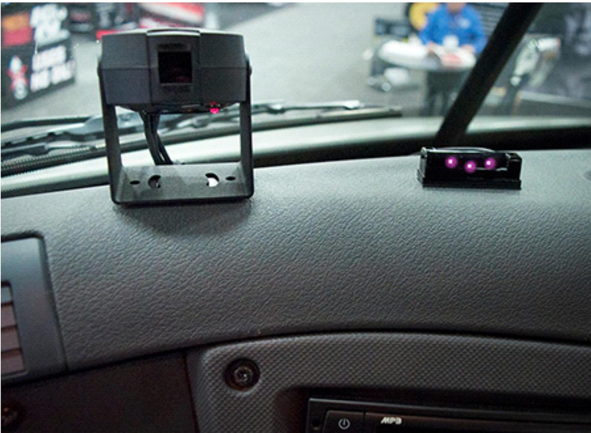
Guardian system in truck cab to detect fatigue and distraction.
