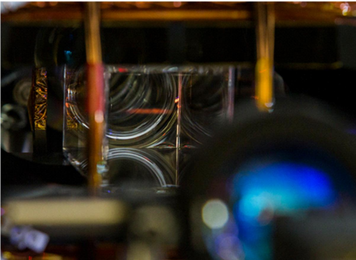
The machine that brought a pulse of laser light to a standstill, trapping the photons inside a four-centimetre-wide cloud comprising billions of super-cold rubidium atoms – a phenomenon called 'stationary light'.
